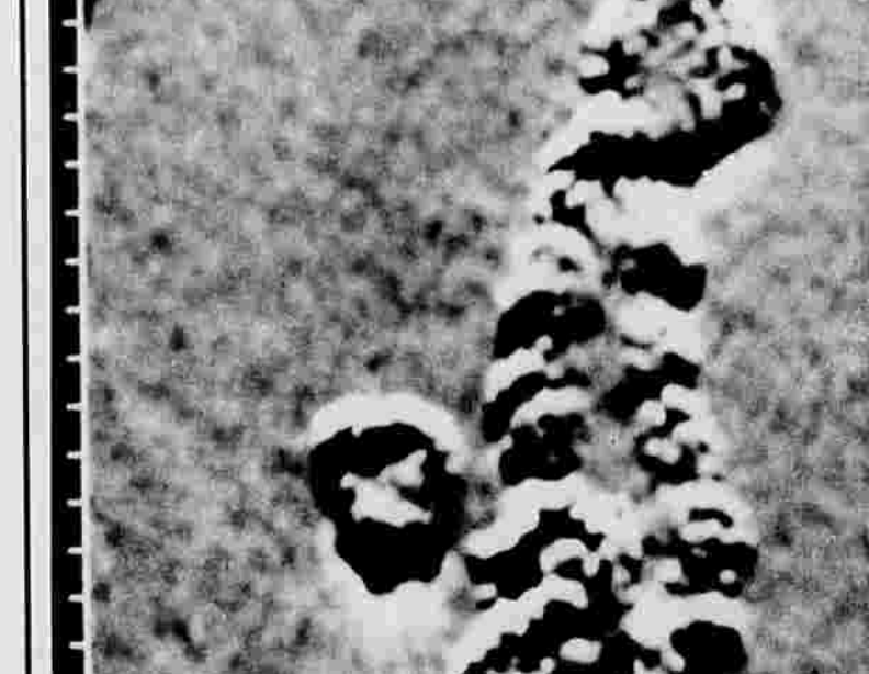
DNA HELIX IMAGE — This is one of the first images of individual lengths of native DNA, showing the double helix, obtained by scientists from Lawrence Livermore National Laboratory and Lawrence Berkeley Laboratory. The three-dimensional image, magnified one million times, was made through a scanning tunneling microscope. The images support recent evidence that DNA exists in several different variations of its helically wound shape.
